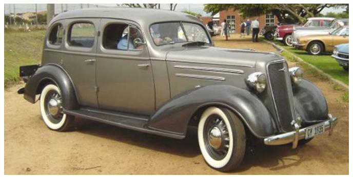
which open at the forward edge of the door instead of the usual back edge—while only the rear doors on the Standard are this design. The roof of the Master is the innovative "turret-top," which is more rounded and fabricated with a single piece of metal. The square top of the Standard was built with wood or fabric at the seams which had a tendency to rattle after a while, causing a lot of noise.
